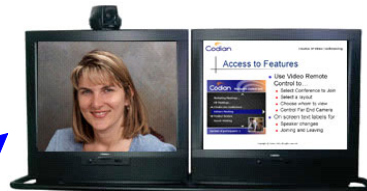
H.239 capable endpoint receives dual-stream image
