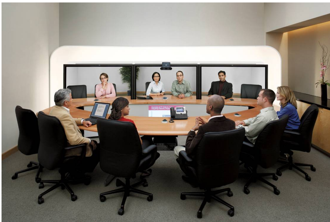
TelePresence System 3000. The data collaboration screen is below table in front of speaker system. Camera unit on center screen is a few inches down from top level and houses three 1080p cameras. Microphones are table-top and user interface is IP phone.
